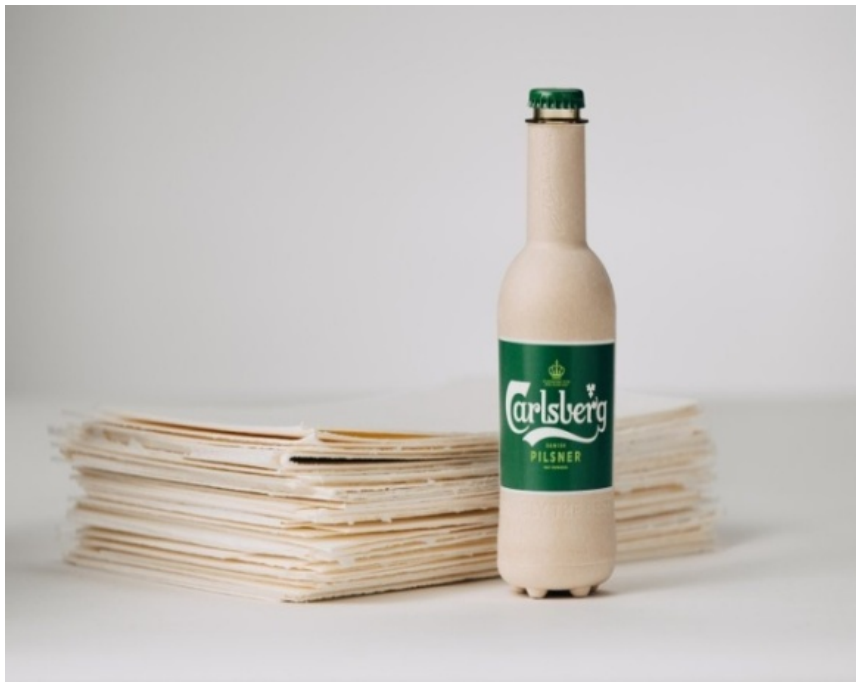
Fig. 1 Samples made by Sugarcane fiber & Casein
